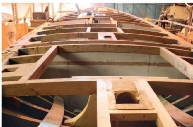
Deckbeams, thwartships, and carlins, fore-and-aft around cut-out areas
