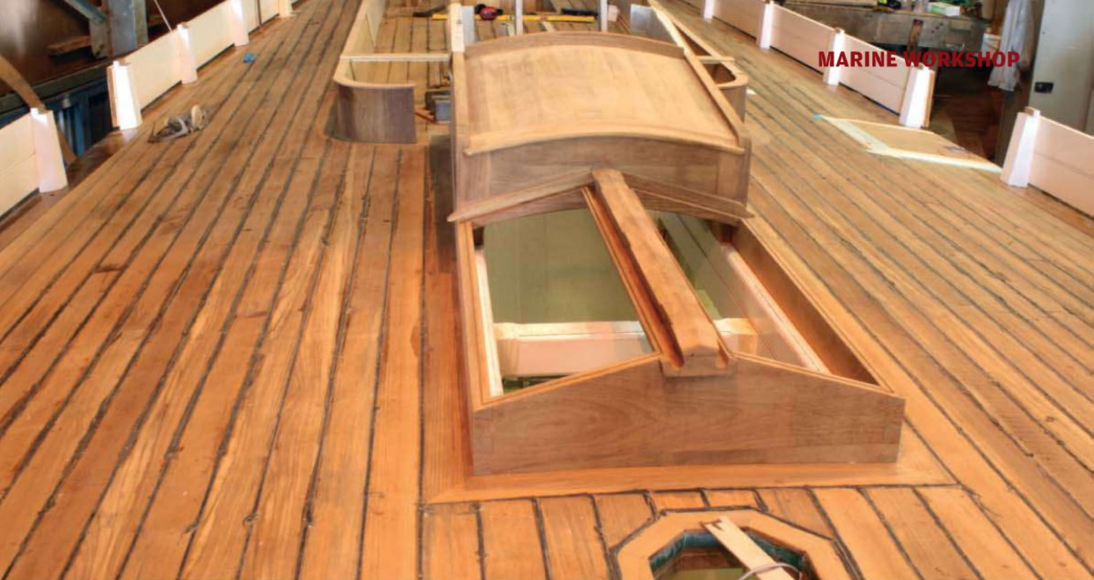
Above: The teak deck, with mast aperture, skylight frame, hatch, coamings and bulwarks
