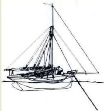
1 The Smack anchors and the baulks are lowered over the starboard side by the baulk tackle. The handfleets have been taken round the bow and shackled by the stringer into the cable
