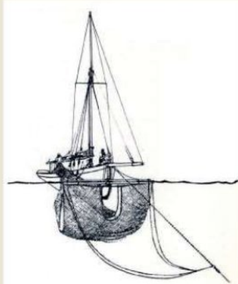
3 The gear aforehead. Once the templines are adjusted, the lower baulk will be dropped on the wind chain and the net paid out on the tide
