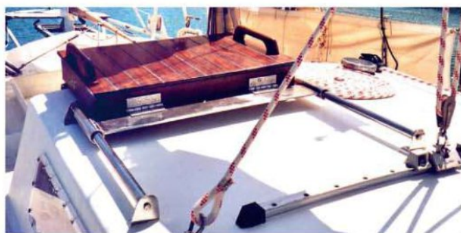
Left: The new hatch in the closed position viewed from ahead. Right: The new hatch in the open position taken from the same angle. The hinges allow the hatch to lift until it clears the coamings, allowing it to slide open
