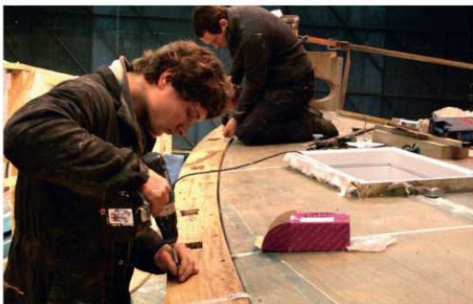
Above: The teak deck, with mast aperture, skylight frame, hatch, coamings and bulwarks
